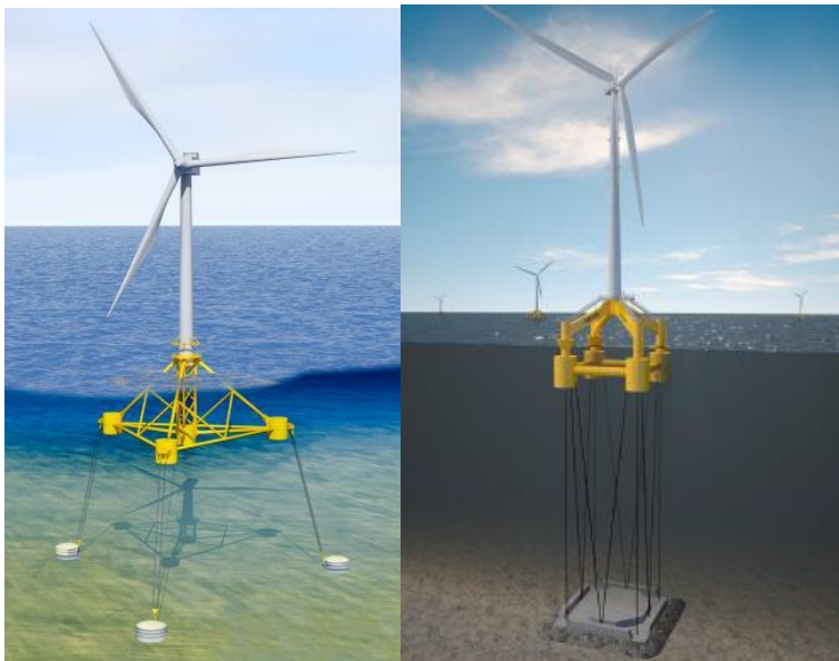
Plate 3.1 Indicative tension leg floating platforms
